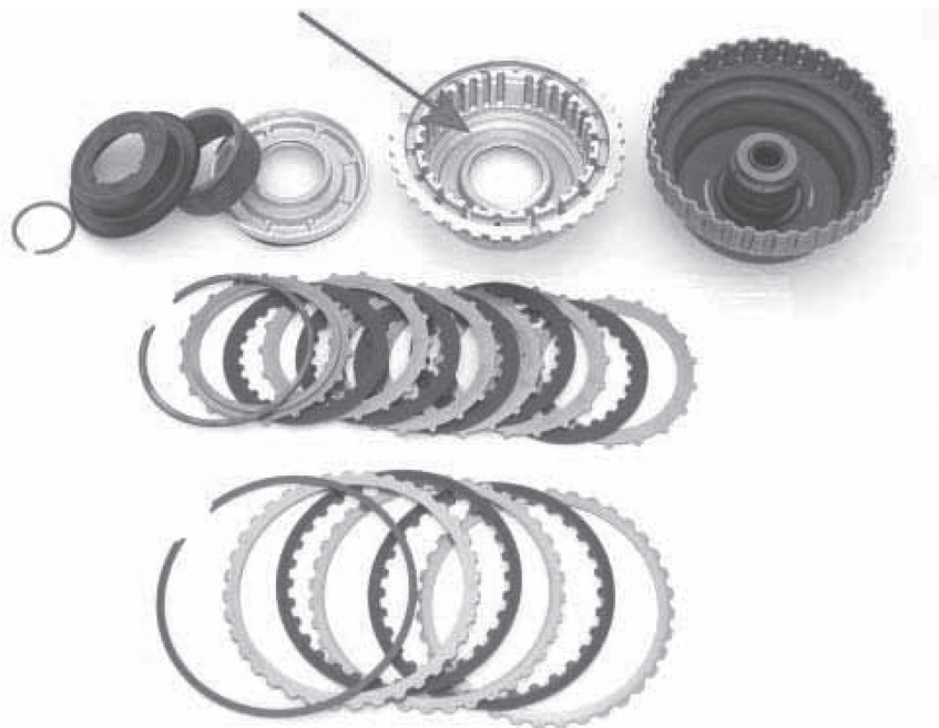
Check for cracks in this area
